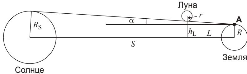
$$h_L = R + r + \alpha \cdot L = R + r + \frac{R_S - R}{S} \cdot L = \frac{R_S L + R(S - L) + rS}{S} = 9950 \text{ км.}$$
